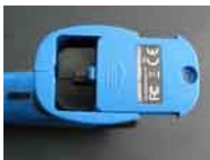
6. Remove the battery cover
