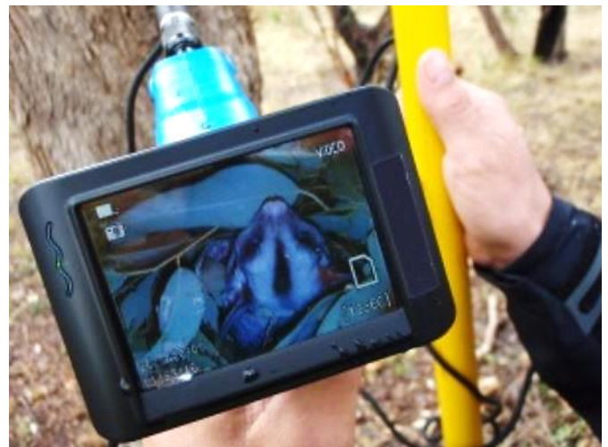
A pole mounted camera with a separate screen which allows ground-based nest box inspection (Photo: Treetec)
