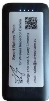
**CHARGING:** Connect a 5 volt/ 2 amp phone charger to the **USB micro** socket labelled **IN** on the top of the Smart battery. Charging is automatic; blue leds indicate progress, when fully charged 4 blue leds are lit. Charge time is around 3~4 hours.
