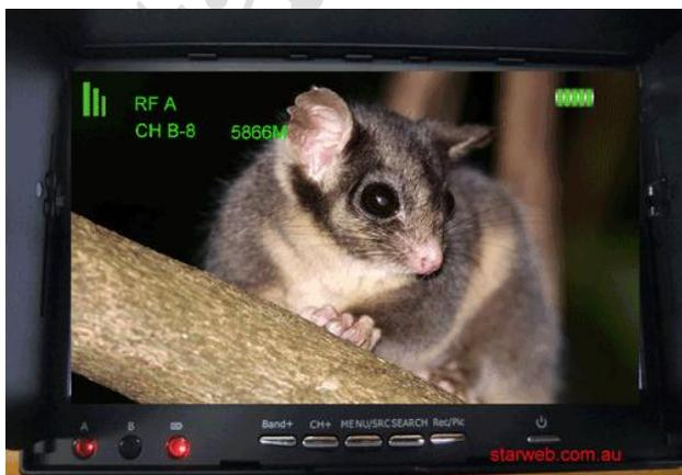
Monitor requires the two antennas. Open the sun shade, press the **POWER** button once, red led **A** will light & the LCD Monitor will come ON. Live video from the inspection camera should be visible on the LCD screen. Multiple LCD Monitors can view the live video from a single Nest box Camera.
