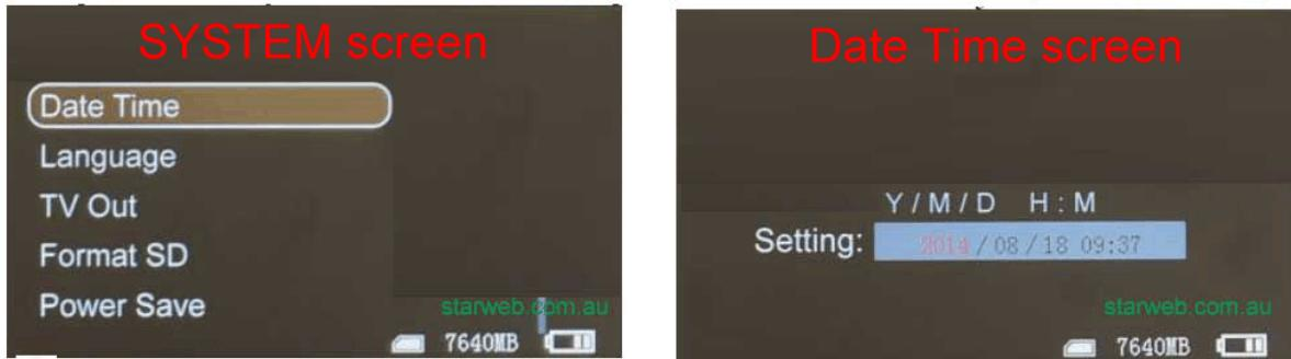
The display format is – Year – Month – Date – Hour – Minutes - Seconds. The editable option will be highlighted in red. Use buttons 1 & 2 to increase or decrease the count then press button 5 to accept the change & move to the next option. Repeat the procedure for all the options.
