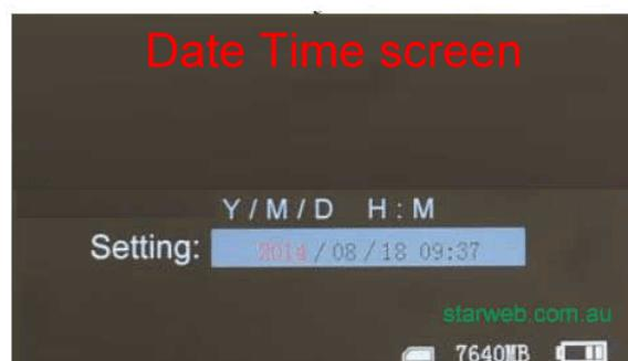
The display format is – Year – Month – Date – Hour – Minutes - Seconds. The editable option will be highlighted in red. Use buttons 1 & 2 to increase or decrease the count then press button 5 to accept the change & move to the next option. Repeat the procedure for all the options.
