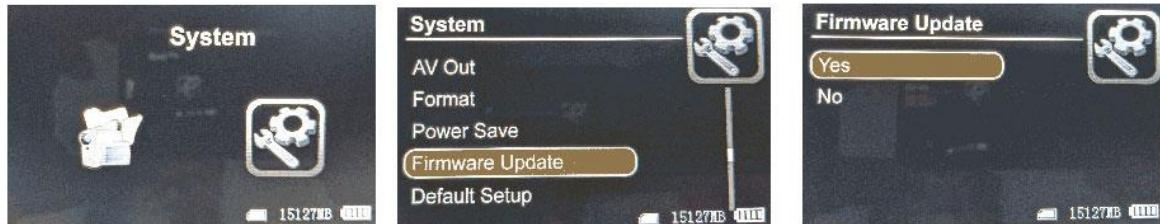
Press button 5 to access the **Firmware Update** screen, then with **Yes** highlighted press button 5 again to start the update. Do not press any other buttons during the update process.
